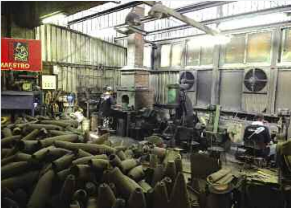
THE MAESTRO WU FACTORY WITH ITS COPIOUS SUPPLY OF STEEL SHELLS. THE WORKER ON THE LEFT IS MELTING A SHELL SECTION IN THE FURNACE, THE STAMPING PRESS IS IN THE CENTRE, WHILE ANOTHER WORKER POLISHES A BLADE.
